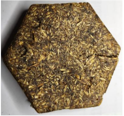
Test article made from 100% bio-epoxy and hemp filler.
